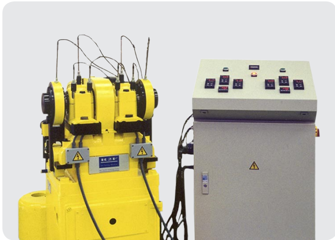
R2F grease test rig
