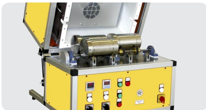
Roll stability test rig
